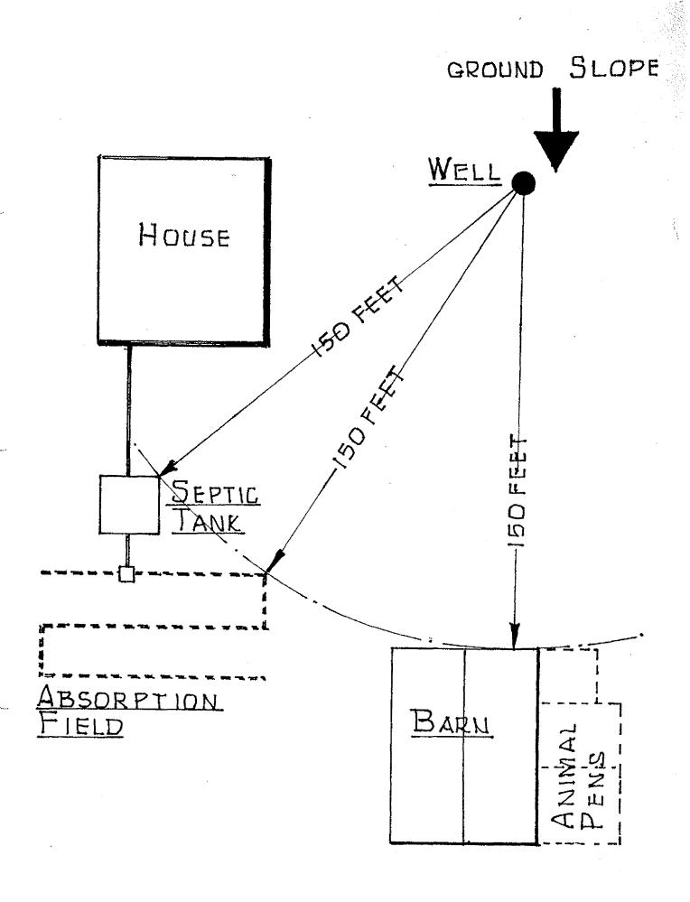
FIGURE 1. PROPERLY LOCATED WELL
